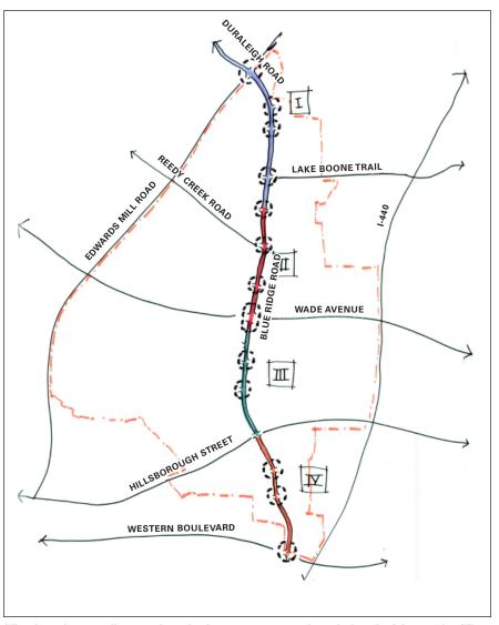
The above diagram illustrates how the character may vary along the length of the corridor. The circles identify key intersections to address for pedestrian mobility.
