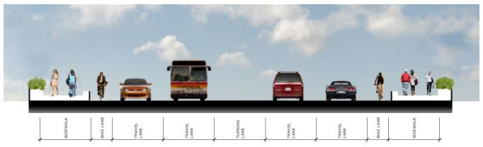
The future bridge cross-section would therefore be expanded (or replaced) to meet a 96-foot minimum width. The existing 70-foot width can be restriped to provide four 11- to 12-foot travel lanes, a 11- to 12-foot center turn lane, and 5-foot bike lanes. This would roughly match Blue Ridge Road on either side of the bridge (the 12-foot lanes on the bridge would ideally be reduced to 11 feet). The bridge would still need widening to add sidewalks.
