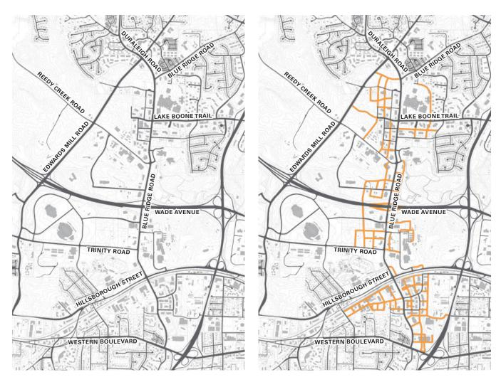
The existing street network (above, left) does not provide enough network to a walkable and sustainable district. The proposed framework (above, right) adds a secondary network of streets to support the development and increase connectivity. A typical street cross-section (to the right) will provide ample facilities for pedestrians, transit, bicycles, and cars.
